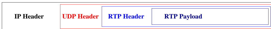
Figure 2.8: IP packet containing real-time data encapsulated in a UDP and RTP packet
